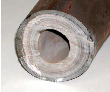
A cross-section of a heat exchanger tube with a thick layer of limescale build-up on the inner wall.
