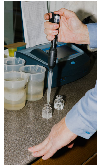
Left: Water analyzing equipment at the Chester Water Authority treatment plant. Right: Water being tested for chlorine residuals.
